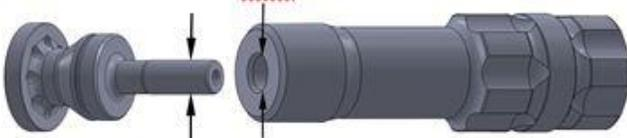
**Clearance 4: Check Valve OD to Air Dist ID .009**
